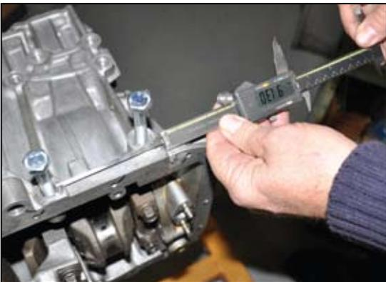
Carefully measure the block to determine the position of the plate mounting holes. Trim the plate to remove any excess material.
