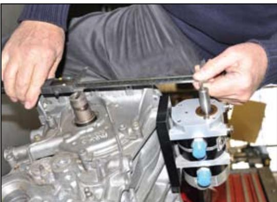
Measure distance from center of pump shaft to the crank centerline. Aviaid will supply the correct belt and pulleys.
