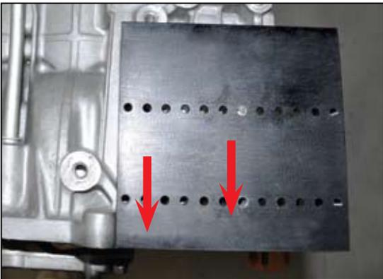
Position the Universal Mounting Plate where you can utilize the pre-drilled holes to mount the pump. Drill holes to attach plate.
