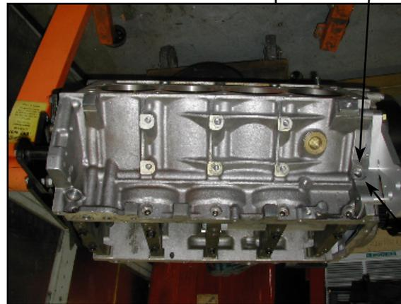
OEM oil filter ports. Front port supplies oil to filter, must be plugged. .510/.518 use 555-074 freeze plug. Rear port from filter to block can supply engine or must be plugged. .545/.550 use 555-092 freeze plug.
