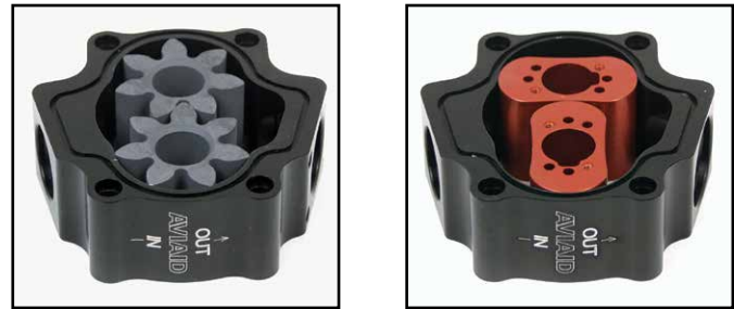
Aviaid Series 2 pumps feature an enlarged 7-tooth gear set on the pressure side and a twin-lobe Roots-type setup in the scavenge sections.
