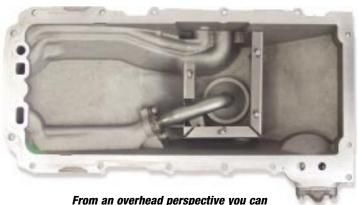
rrom an overnead perspective you can see how the insert "cage" traps the oil around the factory pickup.
