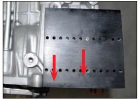
Position the Universal Mounting Plate where you can utilize the pre-drilled holes to mount the pump. Drill holes to attach plate.
