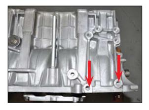
Examine block for logical mounting points. Using two holes that are parallel with the centerline of the crank is preferred.
