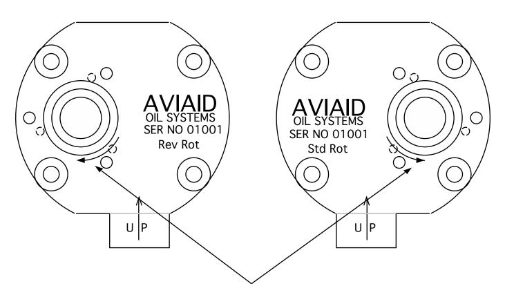
Direction of Drive Shaft Rotation as seen from Regulator end of Pump
