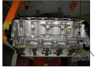
OEM galley port. Transfers oil to rear of block. Passageway must at some point be plugged. 5/8"
