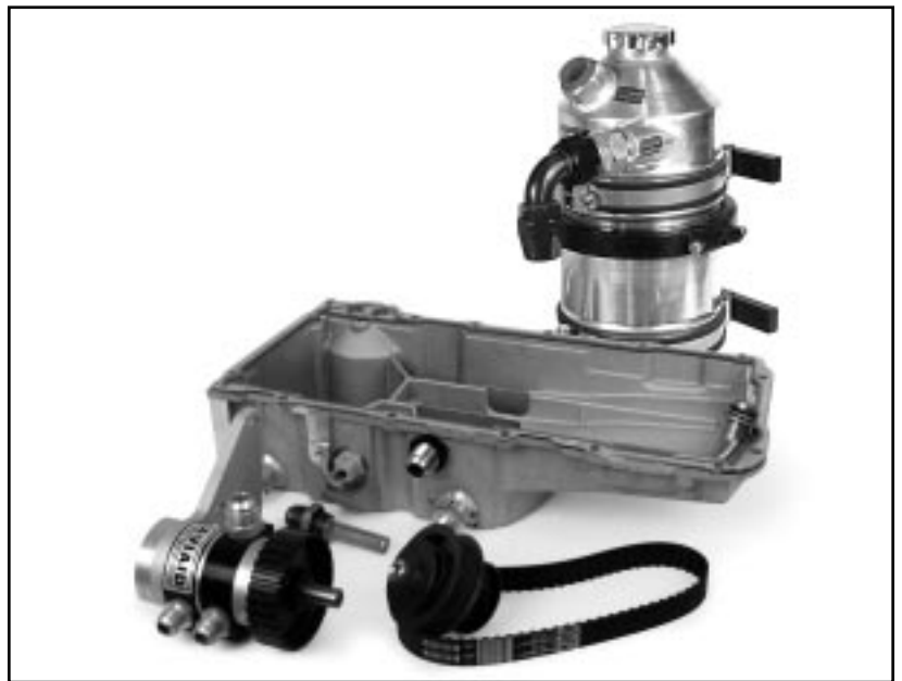
2-section dry sump pump with bracket for mounting to the cylinder head
