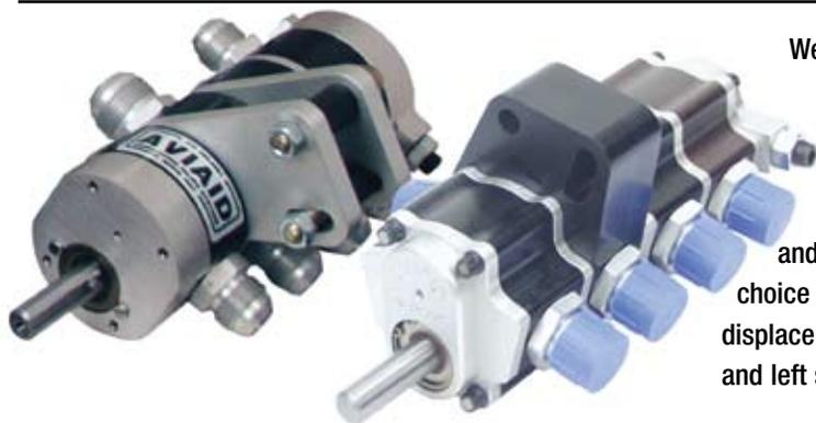
We offer 4-stage pumps in the standard Series 1 and higher performing Series 2 configurations. These include three scavenging and one pressure section. Pump choice is relative to engine displacement and modifications. Both right and left side mount setups are offered.
