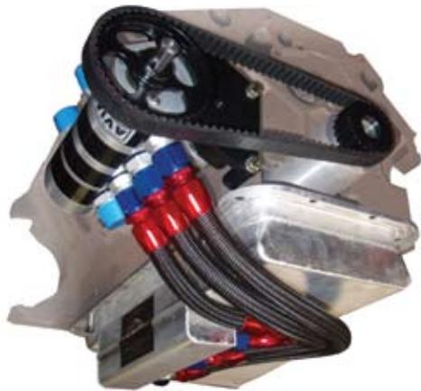
Aviaid has developed mounts that attaché to either the left or right side of the block and allow the pump to be driven from the back side of the damper through use of a special damper sleeve for the HTD drive.
