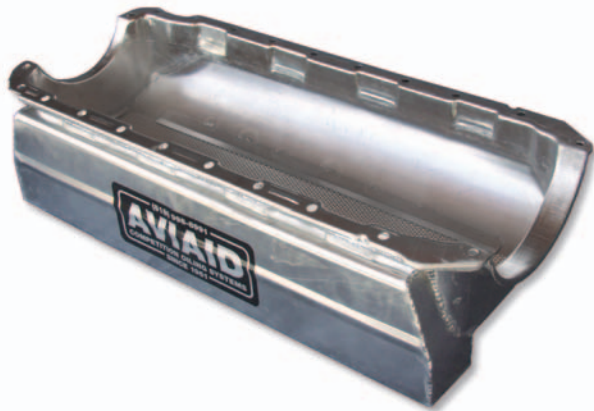
52210 BBC 3 pickup left side outlet dry sump pan for left side mount installation.
